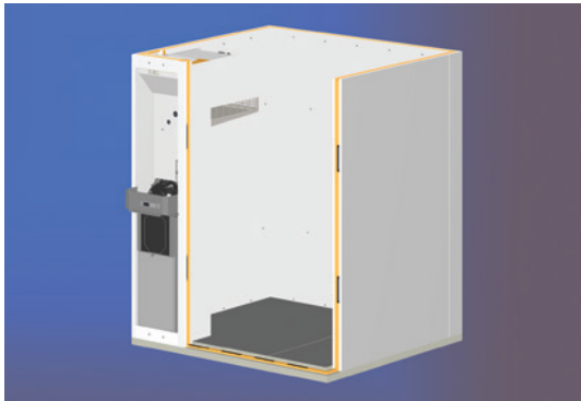
Fig. 9. The assembly of the wall panels
